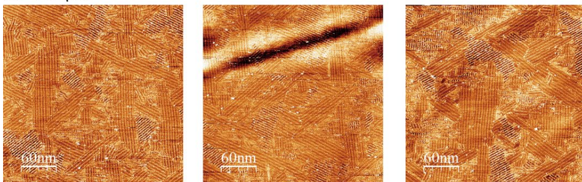
Figure S7. Representative STM images of 1-Fb at different concentration at mixed solvent of OA/PO = 0.5/99.5 (v/v)–HOPG interface ( I_{\text{set}} = 20 \text{ pA} , V_{\text{bias}} = -800 \text{ mV} , 300 \times 300 \text{ nm}^2 ). The concentration of 1-Fb was (a) 25 \mu\text{M} , (b) 75 \mu\text{M} , (c) 100 \mu\text{M} , and (d) 150 \mu\text{M} respectively. The statistical data to determine the averaged surface coverage of 2D ordering at a concentration was summarized in Table S7.
