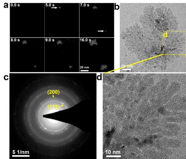
**Figure S1.** (a) Formation process of Pd nanodendrites using an electron dose rate of  $2.37 \times 10^3 \text{ e/nm}^2\text{-s}$ ; (b-d) Ex situ TEM image and selected area electron diffraction and high resolution TEM images of Pd nanodendrites synthesized in a liquid cell.
