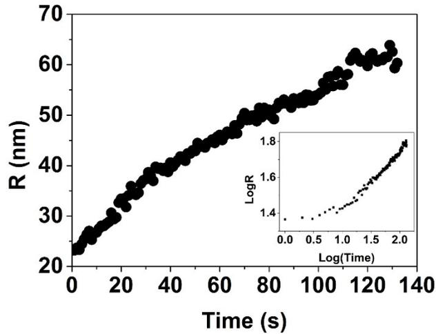
**Figure S5.** Radius of the fractal-like island nanocrystals (Figure 3a in main text) as a function of growth time at 1 mM precursor concentration using an electron dose rate of  $4.47 \times 10^3 \text{ e/nm}^2\text{-s}$ .
