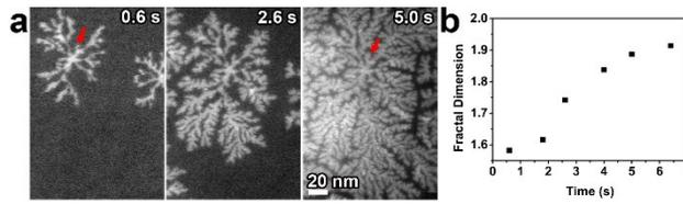
**Figure S4.** Electron dose rate effects on the Pd nanodendrite growth process. (a) The growth process of Pd nanodendrite using an electron dose rate of  $6.71 \times 10^4 \text{ e/nm}^2\text{-s}$ ; (b) Fractal dimension of Pd nanodendrite as a function of time.
