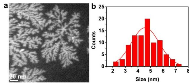
**Figure S2.** Branch width of nanodendrites. (a-b) HAADF STEM image of nanodendrites and a corresponding histogram of dendritic branches width distribution.
