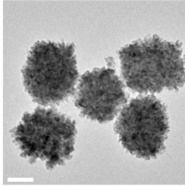
**Figure S7.** TEM image of Pd island-like nanocrystals synthesized in flask. Scale bar: 50 nm.
