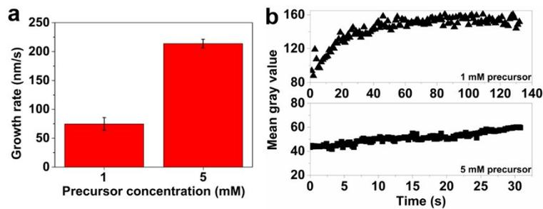
**Figure S6.** Differences of growth rate and contrast of Pd nanocrystals during growth process: (a) Different growth rates are showed at 1.0 mM and 5.0 mM precursor concentration using an electron dose rate of  $4.47 \times 10^3$  and  $1.12 \times 10^3 \text{ e/nm}^2\text{-s}$ , respectively; (b) Difference of contrast evolution of Pd nanocrystals at 1.0 mM and 5.0 mM precursor concentration using an electron dose rate of  $4.47 \times 10^3 \text{ e/nm}^2\text{-s}$ .
