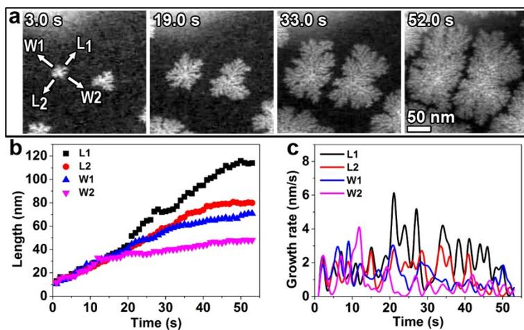
**Figure S8.** Influence of adjacent nanodendrites on the of growth process of Pd nanodendrites. (a) A time lapse series of HAADF-STEM images at an electron dose rate of  $2.37 \times 10^3 \text{ e/nm}^2\text{-s}$ ; (b) Nanodendrites length and (c) growth rates along different directions.
