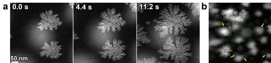
**Figure S9.** (a) Pd nanodendrites formation process closing to the two  $\text{Si}_3\text{N}_4$  membranes using an electron dose rate of  $9.46 \times 10^3 \text{ e/nm}^2\text{-s}$ . (b) Overlapped nanodendrites in liquid cell. Scale bar: 100 nm.
