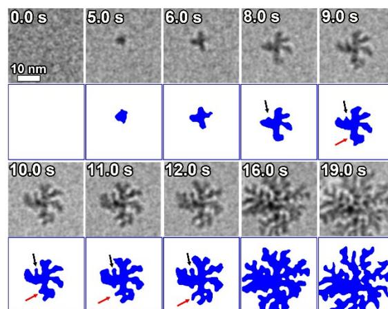
**Figure S3.** TEM image series show that a nanocluster ( $\sim 5 \text{ nm}$ ) first form and then grow into nanodendrite.
