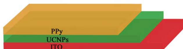
Scheme S1 Schematic representation of the structure of the PPy/UCNPs photoelectrode.
