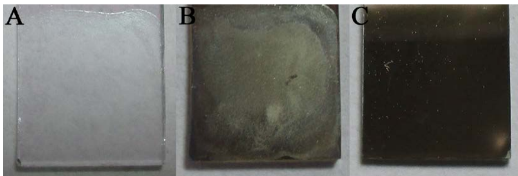
Fig. S2. Photographs of (A) UCNPs; (B) UCNPs/PPy; (C) PPy on the ITO (1cm × 1cm).
