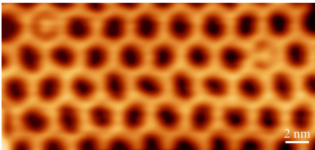
Figure S3. STM images taken after annealed at 200 °C with 1.0 °C/min rate for deposition of TBB onto Ag(111) held at RT ( V = 1.0 V, I = 500 pA) .
