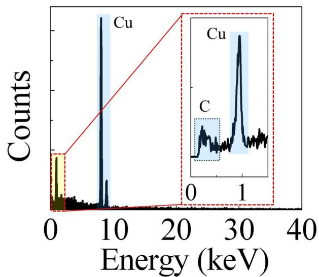
Figure s4. Typical X-ray energy dispersive spectrum (EDS) pattern obtained from the sample. Inserted figure is a magnified region (shaded with yellow) of the EDS spectrum as indicated.
