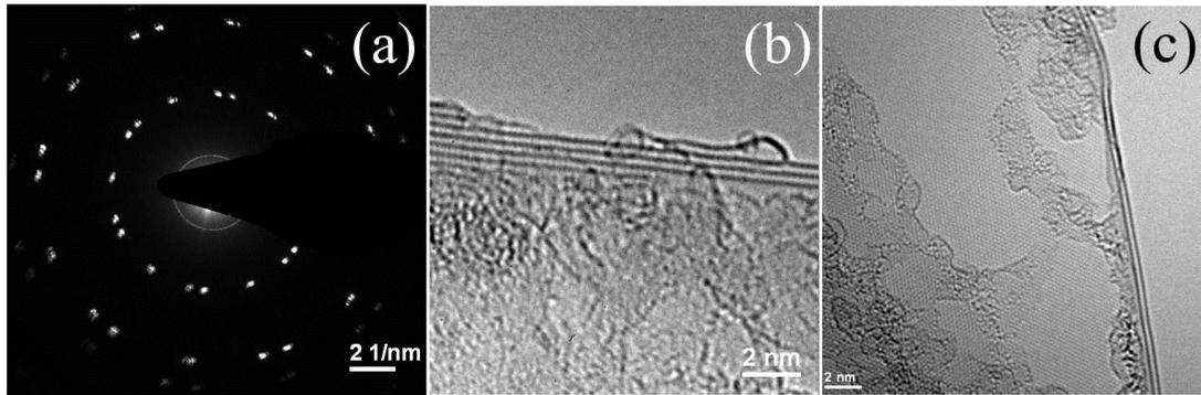
Figure s1. (a) SAED pattern of the graphene structure. The splitted diffraction spots indicate the multilayer nature of the sample. And typical TEM images obtained at the edge of the multilayer graphene structure: (a) normally observed thick region with layer  $> 3$ ; (b) thin region with a double layer structure.
