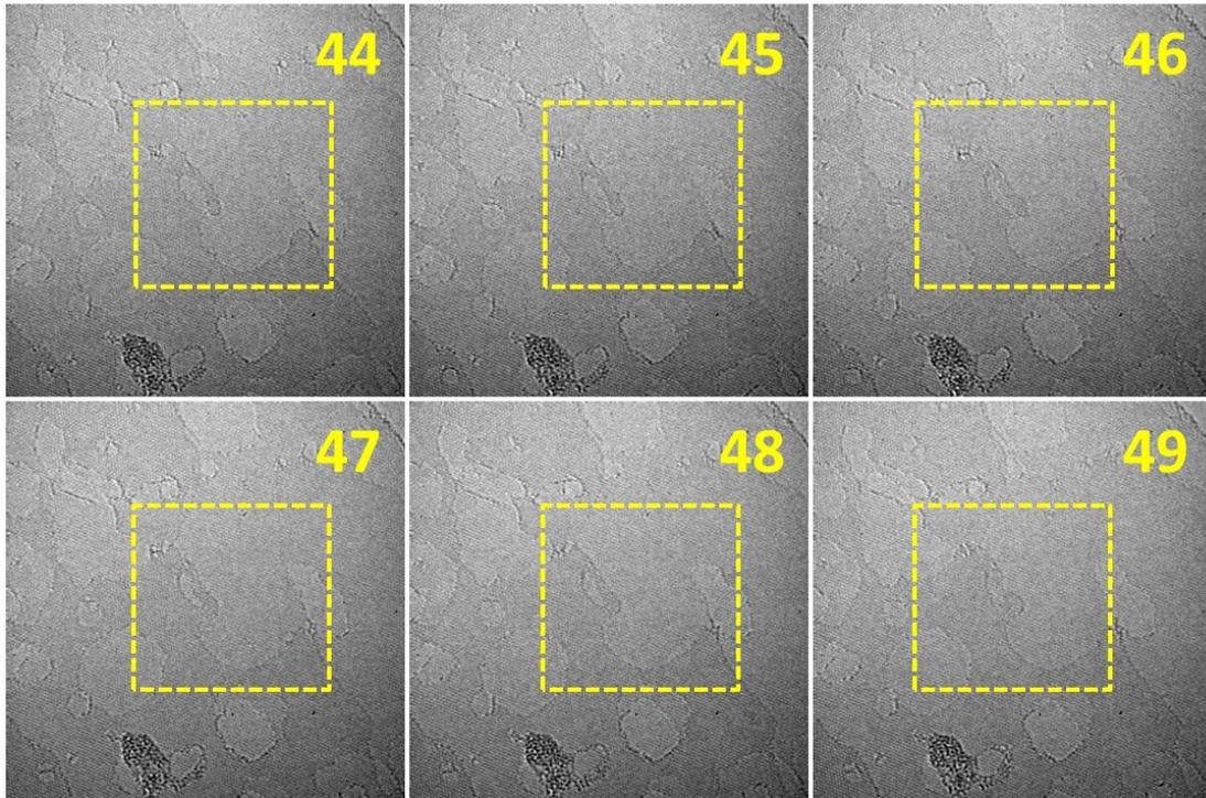
Figure s2. (Continued) Detailed TEM image sequence shows the re-orientation, alignment and merging of the GFs. Yellow dashed rectangular highlight the interested region. Numbers is the sequence of the image frame.
