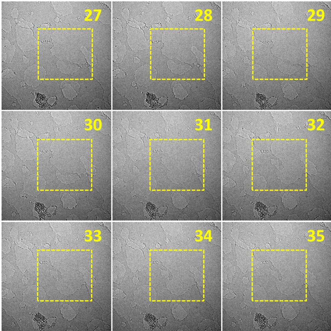
Figure s2. (Continued) Detailed TEM image sequence shows the re-orientation, alignment and merging of the GFs. Yellow dashed rectangular highlight the interested region. Numbers is the sequence of the image frame.
