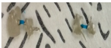
Scheme S1: Illustration of fabrication of a simple device for I-V electrical measurements on a glass slide.
