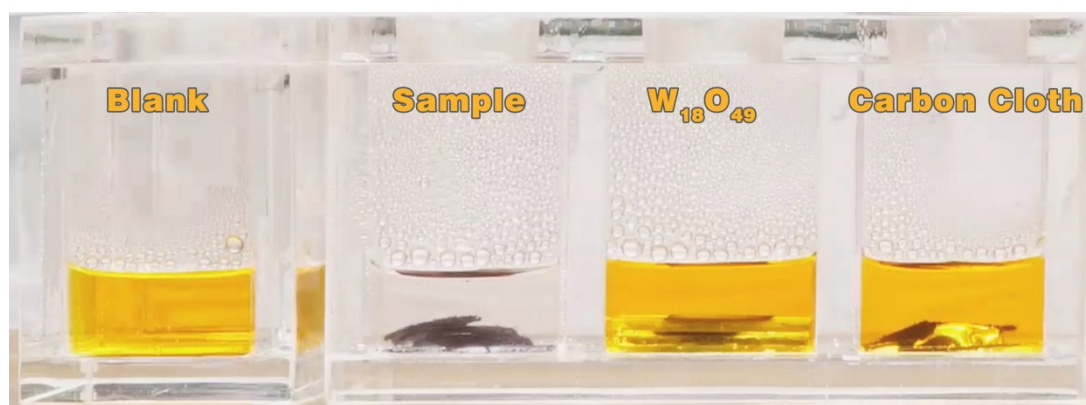
Supplementary Fig.7 Degradation of the MO solution using different nanostructures under sunlight irradiation, where Sample denotes the fabricated W 18 O 49 /WO x /W dendritic nanostructure. (a) Before degradation; (b) After degradation for 1.5 h.
