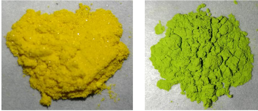
Fig. S3. Images for powder of the as synthesized and dehydrated phase of (\text{bix})\text{CuCl}_4 \cdot \text{H}_2\text{O} .
