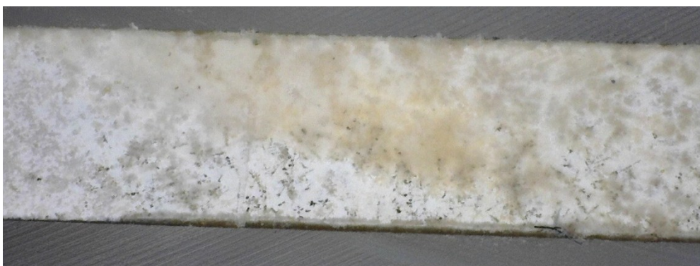
Fig. S12: Ag sealant migration in dual-phase membranes. \text{Al}_2\text{O}_3 pellet membranes with 0 mol% Ag doping operated at 650 °C shows evidence of Ag dendrites within the cross-section of the membrane. Feed-side inlet: 50 mol% \text{CO}_2 , 25 mol% \text{O}_2 and 25 mol% \text{N}_2 . Permeate-side inlet: Ar.
