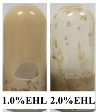
Figure S2. The appearances of the HIPEs stabilized by different EHL concentrations at 3.5 wt% APG, 80 vol% oil and water phase pH of 7.0.
