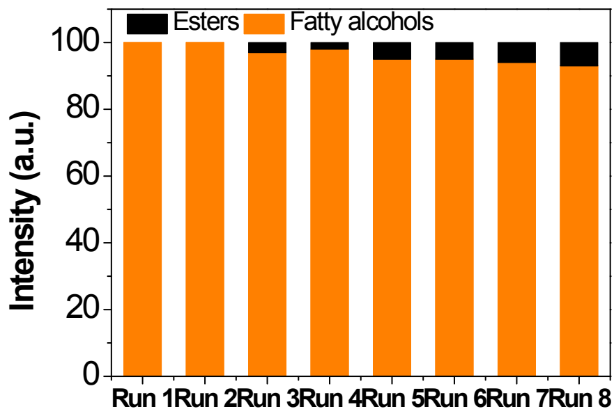
Fig. S15 Recycling test of hydrogenation of algae oil over RuSn/N-C catalyst (treated by sequential hydrogen reduction). Reaction conditions: algae oil (1.0 g), RuSn/N-C (0.3 g), water (80 mL), 140 °C, 6 h, H 2 (5 MPa), stirring at 500 rpm.
