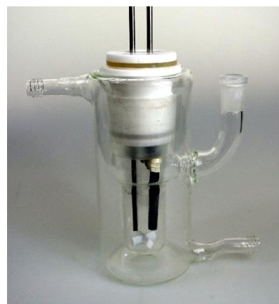
Figure S1 View of an undivided beaker-type cell of 25 mL.
