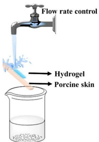
Figure S17. Schematic diagram of impact force calculation by water flow.
