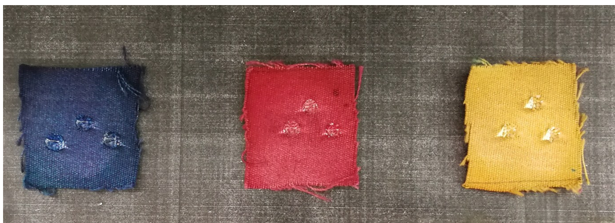
Fig. S18. The optical photographs of water on dyed fabric with self-healing function.
