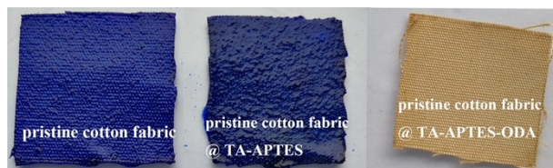
Fig. S15. The optical photographs of pristine cotton fabric, pristine cotton fabric @ TA-APTES and pristine cotton fabric @ TA-APTES-ODA after being soaked into the water dyeing with methyl blue. The superhydrophobic fabric shows excellent anti-fouling behavior.
