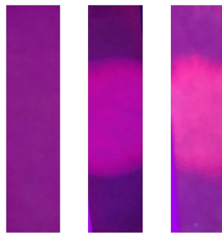
Fig. S4 Detection of albumin through strip test in the presence of UV light (365nm). Changes can be seen post addition of albumin
