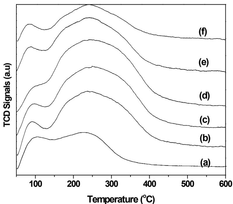
**Figure S.3:** NH<sub>3</sub>-TPD profiles of pure and tungstated TiP catalysts. (a) Pure TiP (b) 5 wt% WO<sub>x</sub>/TiP (c) 10 wt% WO<sub>x</sub>/TiP (d) 15 wt% WO<sub>x</sub>/TiP (e) 20 wt% WO<sub>x</sub>/TiP (f) 25 wt% WO<sub>x</sub>/TiP.
