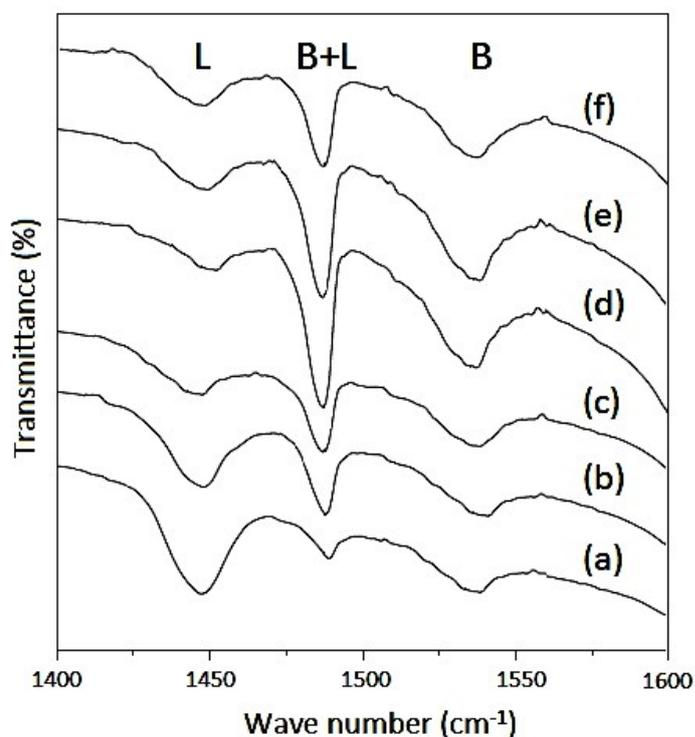
**Figure 7.6:** FT-IR Pyridine adsorption profiles of pure and tungstated TiP catalysts.
