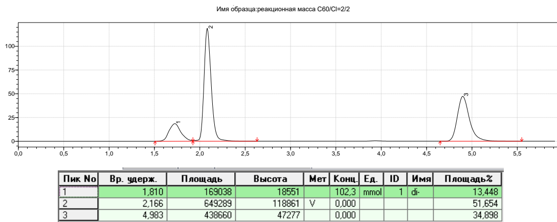
Fig. S7 HPLC data for the reaction of C 60 with 2-(4-chloro-3-oxo-1-phenylbutan-2-yl)isoindoline-1,3-dione ( Cl-K ) in toluene/acetonitrile (1:1).
