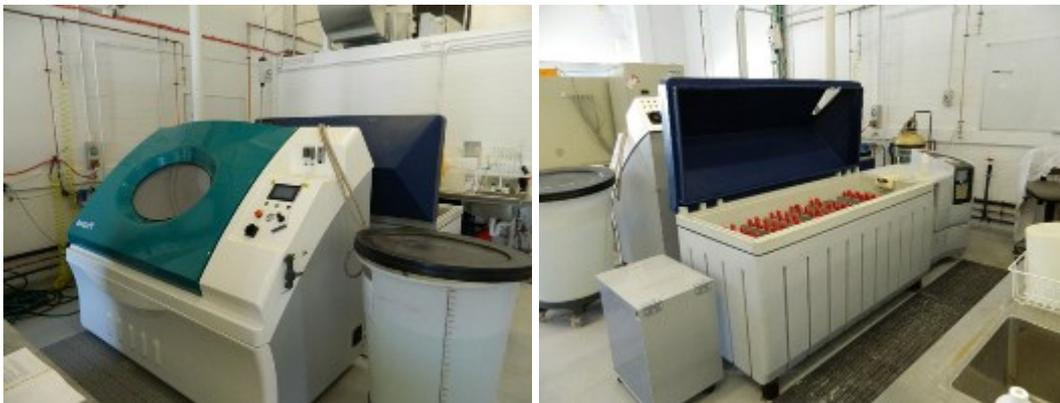
**Figure S6.** The Neutral Salt Spray Chambers located and used at CSIRO Clayton for tests.
