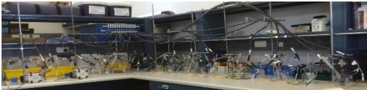
**Figure S5.** Image of current CSIRO HTP electrochemical assay used to evaluate single compounds and mixed inhibition compound systems for corrosion inhibition activity.
