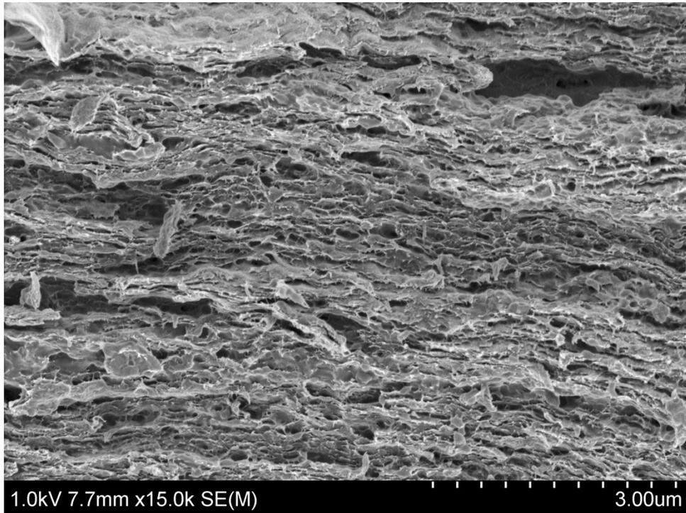
**Figure S2:** SEM image of cross-section from tensile testing of a composite CNF-PBMA<sub>82</sub> treated only at room temperature.
