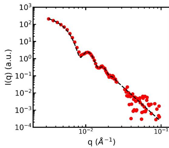
**Figure S3:** SAXS form factor of PMMA<sub>100</sub> NPs in dilute aqueous solution. SAXS was performed on the Columbia SAXSLAB equipment and background subtracted. The pattern was fit with a spherical form factor with a radius of 52 nm and a polydispersity of 0.09.
