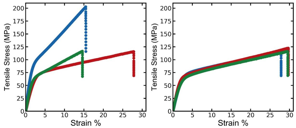
**Figure S1:** Representative curves from *ex situ* tensile testing of (A) CNF reference (blue), CNF-PMMA<sub>100</sub> (red), and CNF-PBMA<sub>82</sub> (green). (B) Three consecutive tests of CNF-PMMA<sub>100</sub>.
