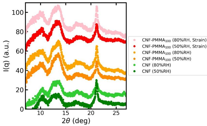
**Figure S6:** Wide angle X-ray scattering performed on CNF and CNF-PMMA<sub>100</sub> at different humidities and under in situ strain.
