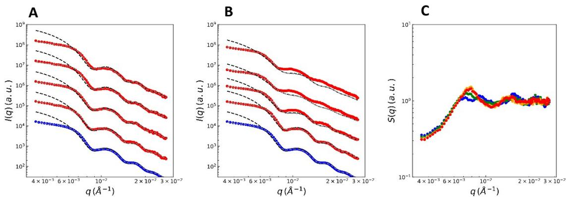
**Figure S7:** Fitting of the SAXS data for CNF-PMMA<sub>100</sub> sample for in situ strain at 50% humidity integrated (A) vertically and (B) horizontally. Blue curves are integrated isotropically. Black dashed lines are form factor fits of the NPs. Grey dashed lines are fits incorporating a Percus-Yevick structure factor. Dividing the data in (A) by the form factor gives (C) the structure factor of the NP scattering.
