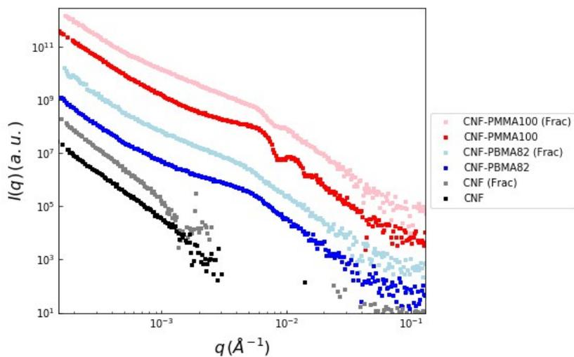
**Figure S5:** Ultra small angle x-ray scattering performed on CNF, CNF-PMMA<sub>100</sub>, and CNF-PBMA<sub>82</sub> before and after strain to failure (“Frac”). The smearing of the pattern in the form factor region of the sample is similar to that seen in the *in situ* scattering. The lack of structural anisotropy at low  $q$  is noted, down to  $\sim 4$  micron, for this radially averaged measurement.
