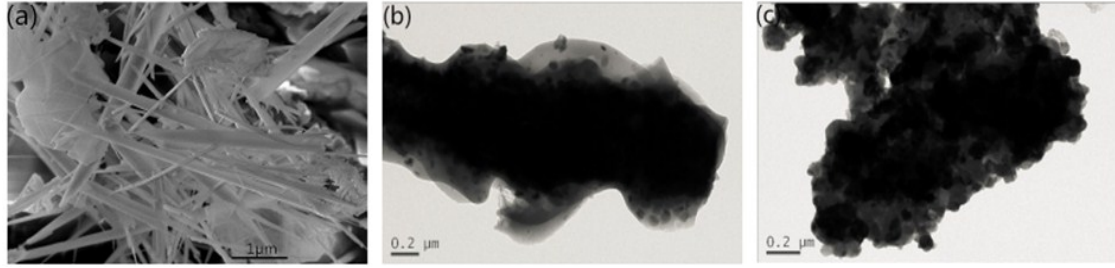
Figure S1. SEM image of (a) Co-N-S-C-700; TEM images of (b) Co-S-C-700 and (c) r-Co-N-S-C-700 (re-activated)
