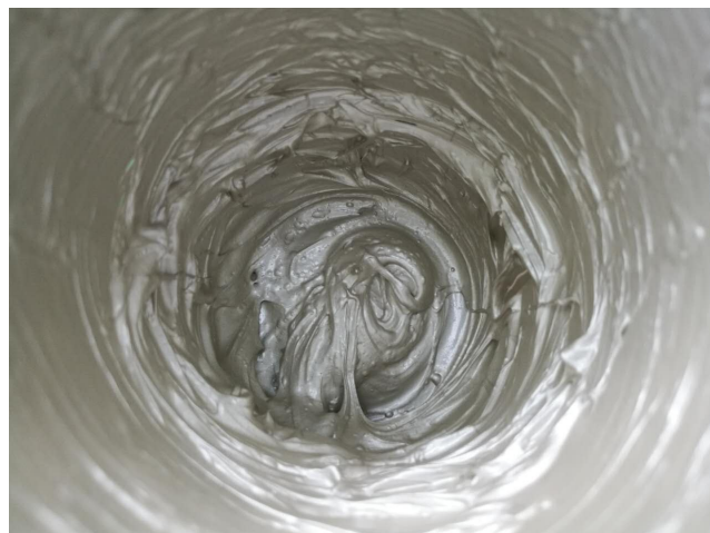
Figure S1. Optical images of solvent-free electrically conductive Ag/EVA composites (filled with 55wt% as-prepared flake silver powders)
