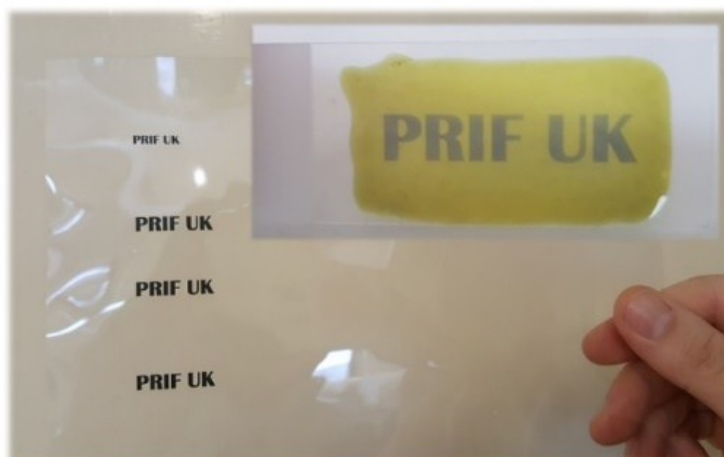
Fig. S31. Logo of our faculty (inset of figure) prepared by irradiation of the blue thin poly (propylene carbonate) film containing Z1 / TBA^+F^- photochromic system with light of 590 nm wavelength through the simple foil photomask.
