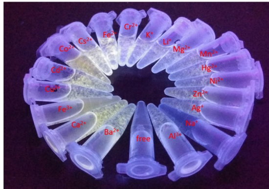
Fig. S11 Photograph of 4 ( 10^{-4} M) upon adding 10 equiv. of various ions in DMSO/ \text{H}_2\text{O} (1:9, v/v) which was observed under a UV-lamp (365 nm).
