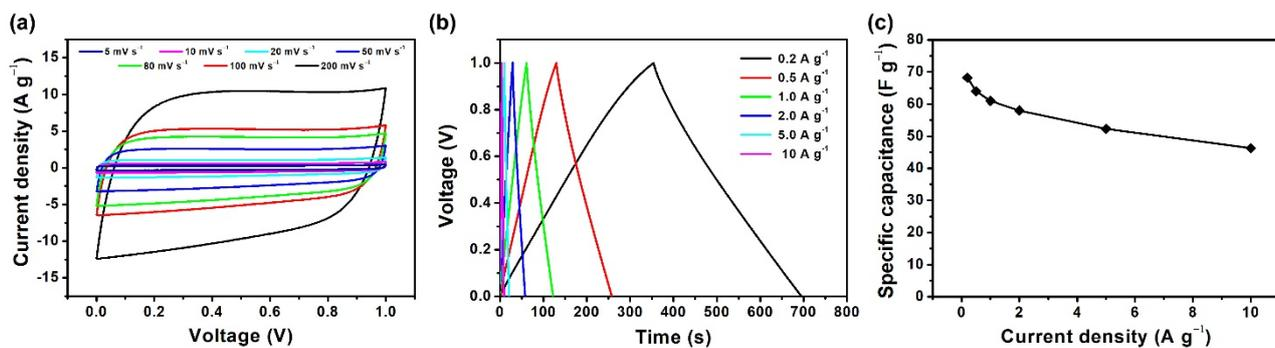
**Fig. S5** (a) CV curves of the ANPC-1-800-0.25//ANPC-1-800-0.25 supercapacitor at different scan rates; (b) GCD curves of the ANPC-1-800-0.25//ANPC-1-800-0.25 supercapacitor at different charge/discharge current densities; (c) specific capacitances of the ANPC-1-800-0.25//ANPC-1-800-0.25 supercapacitor at different current densities. All the measurements were taken in 6 M KOH.
