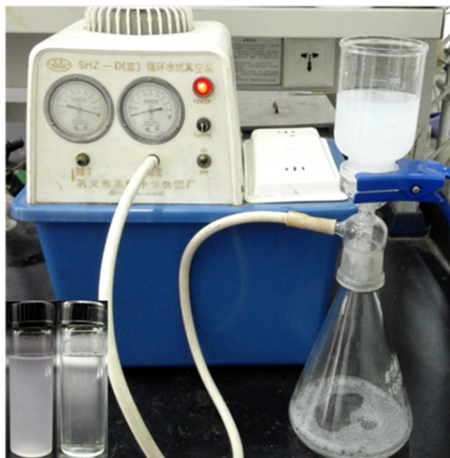
Figure S4. The picture of emulsion separation process, insert image is the emulsion before (left) an after (right) filtration.
