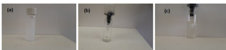
Fig. S3 Separation of surfactant stabilized water in oil emulsion (A) water in oil emulsion, (B) Separation process, (C) Separated oil from water by using the ODTCS-SiO 2 -PP-PU
