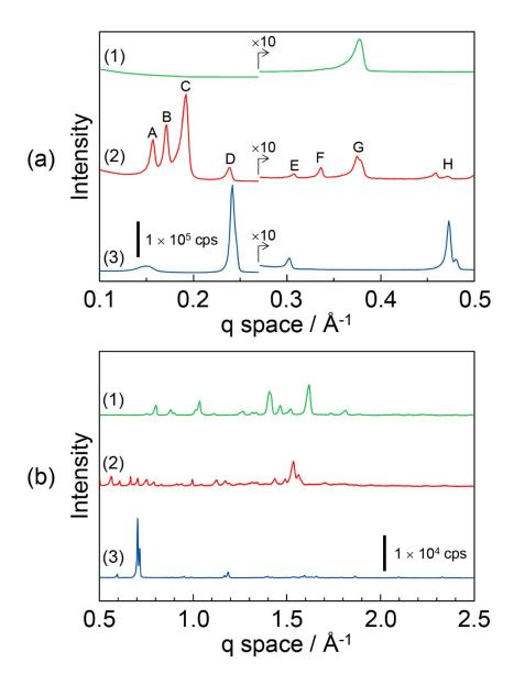
**Figure S1.** The q space  $(2\pi/d\text{-spacing})$  of (1) DOT material, (2) DOT-40 mol% MDP composite material, and (3) MDP material. (a) and (b) show the q space in the low- and high-angle regions, respectively. The q space was calculated from the d-spacing.
