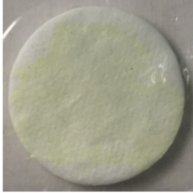
Fig. S2. Digital image of S-GFI film prepared by a dropping-coating method.
