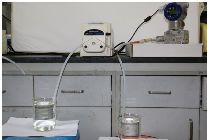
Fig. S4 Filtration procedure used for BSA, SA and HA solutions.
