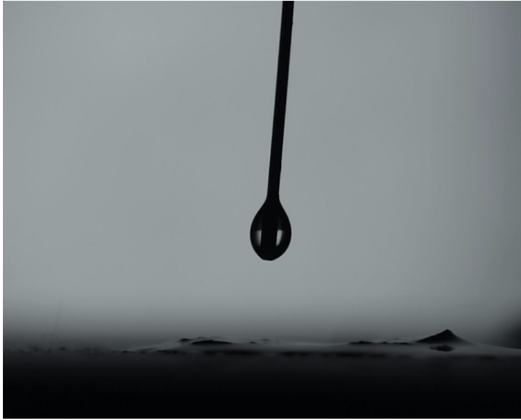
Supplemental Figure S5. Contact angle images between liquid electrolyte and Freestanding TNO/CNFs core/shell arrays
