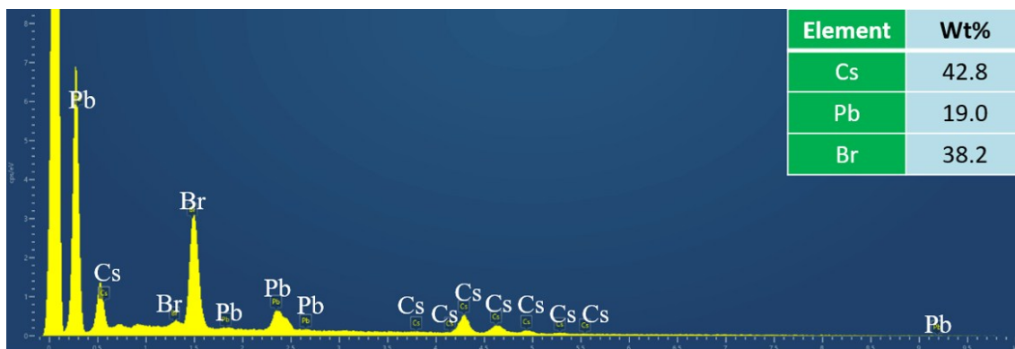
Figure S2. The corresponding EDS spectrum of the shale-like \text{Cs}_4\text{PbBr}_6 perovskite microplates in Figure 1d.
