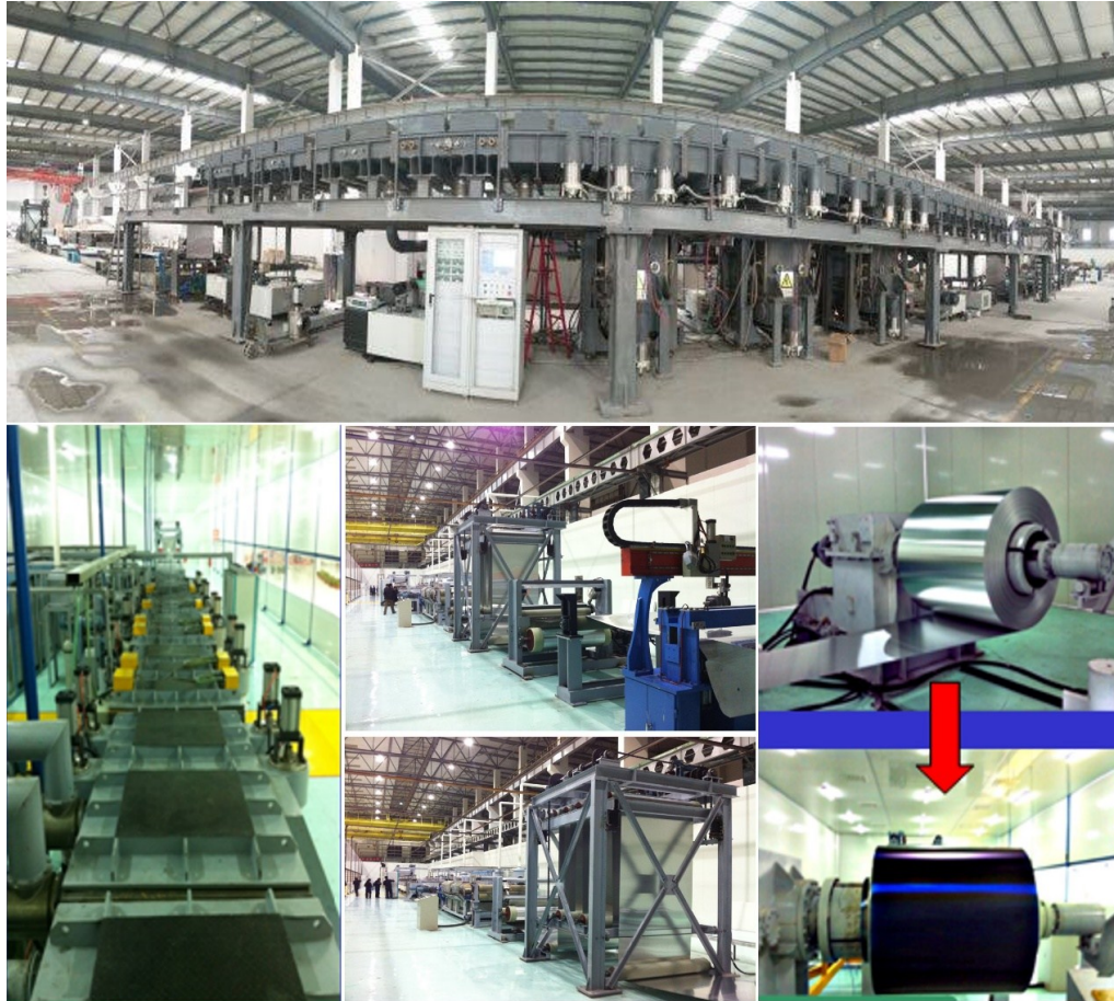
Fig. S12. Photo of the self-developed air-to-air produce line with a length of 90 m and a height of 2.5 m which was used to continuous fabricate large-scale Al–AlN x O y SSACs on Al strip. (a) panoramic photo, (b) overlooking photo, (c, d) panoramic photo from one side, (e) un-winding roller, and (f) re-winding roller.
