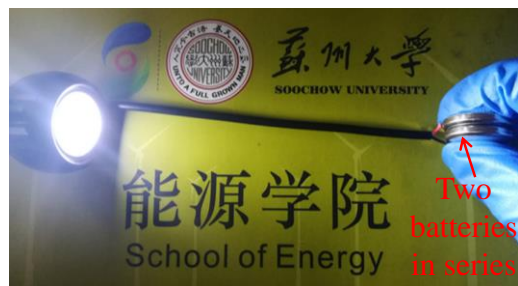
Figure S15. The application of two cycled full NFS@5%CNTs//HC cells for lighting a commercial LED study table lamp.
