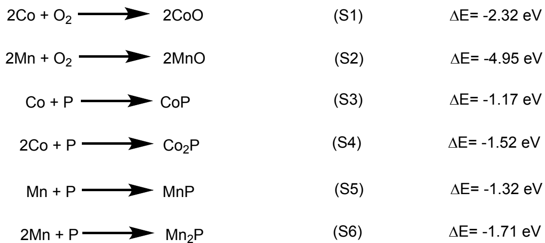
Scheme S2: The calculated reaction energies of formation of CoO, MnO, CoP, Co 2 P, MnP and Mn 2 P, respectively.
