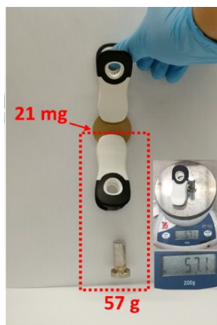
Figure S4. Digital photograph showing the mechanical property of MnOOH@Al 2 O 3 film.
