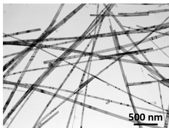
Figure S1. TEM image of MnOOH nanowires.
