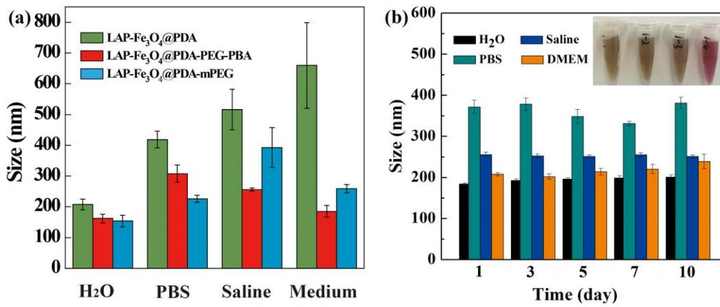
Fig. S7 The hydrodynamic size of (a) LAP-Fe<sub>3</sub>O<sub>4</sub>@PDA, LAP-Fe<sub>3</sub>O<sub>4</sub>@PDA-mPEG and LAP-Fe<sub>3</sub>O<sub>4</sub>@PDA-PEG-PBA in different solvents and (b) LAP-Fe<sub>3</sub>O<sub>4</sub>@PDA-PEG-PBA NPs in different solvents for 1, 3, 5, 7 and 10 days (Images of LAP-Fe<sub>3</sub>O<sub>4</sub>@PDA-PEG-PBA dispersed in water, PBS, Saline and Medium from left to right).
