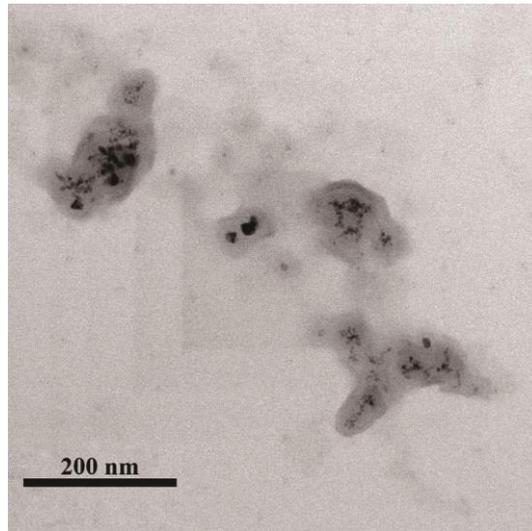
Fig. S4 TEM image of LAP-Fe<sub>3</sub>O<sub>4</sub>@PDA-PEG-PBA NPs in field of 200 nm view.
