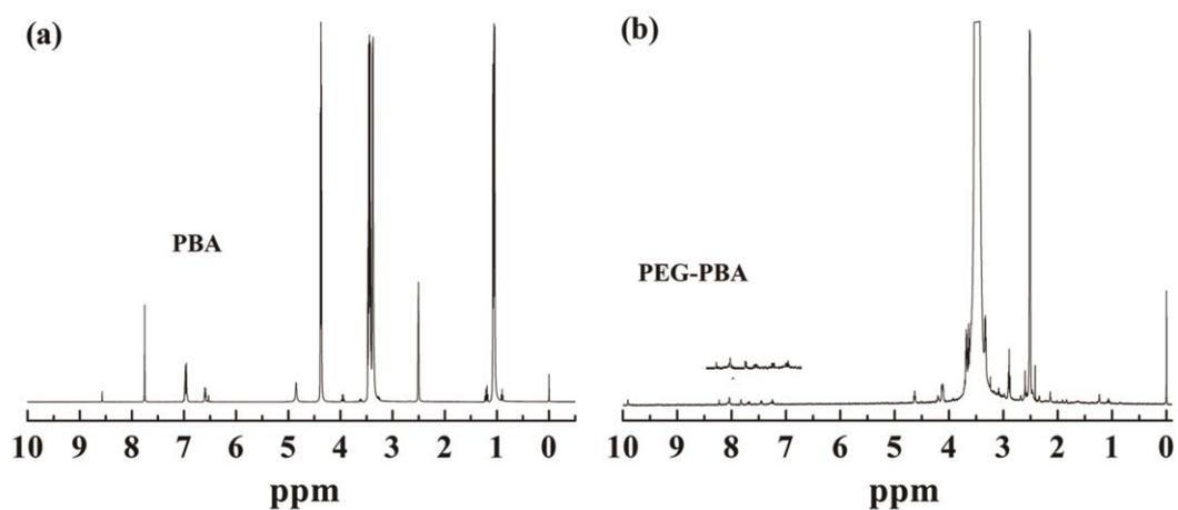
Fig. S3 <sup>1</sup>H NMR spectra of (a) PBA and (b) PEG-PBA.
