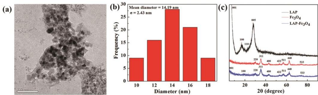
Fig. S1 (a) TEM image and (b) size distribution histogram of LAP-Fe<sub>3</sub>O<sub>4</sub> NPs; (c) XRD patterns of LAP, Fe<sub>3</sub>O<sub>4</sub> and LAP-Fe<sub>3</sub>O<sub>4</sub> NPs.
