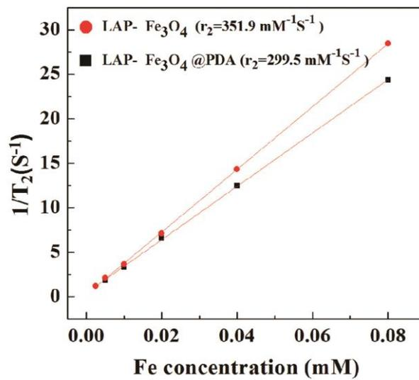
Fig.S8 T<sub>2</sub>-weighted MR linear fitting of r<sub>2</sub> relaxation rate (1/T<sub>2</sub>) of LAP-Fe<sub>3</sub>O<sub>4</sub> and LAP-Fe<sub>3</sub>O<sub>4</sub>@PDA at different Fe concentrations (0.005, 0.01, 0.02, 0.04, and 0.08 mM).
