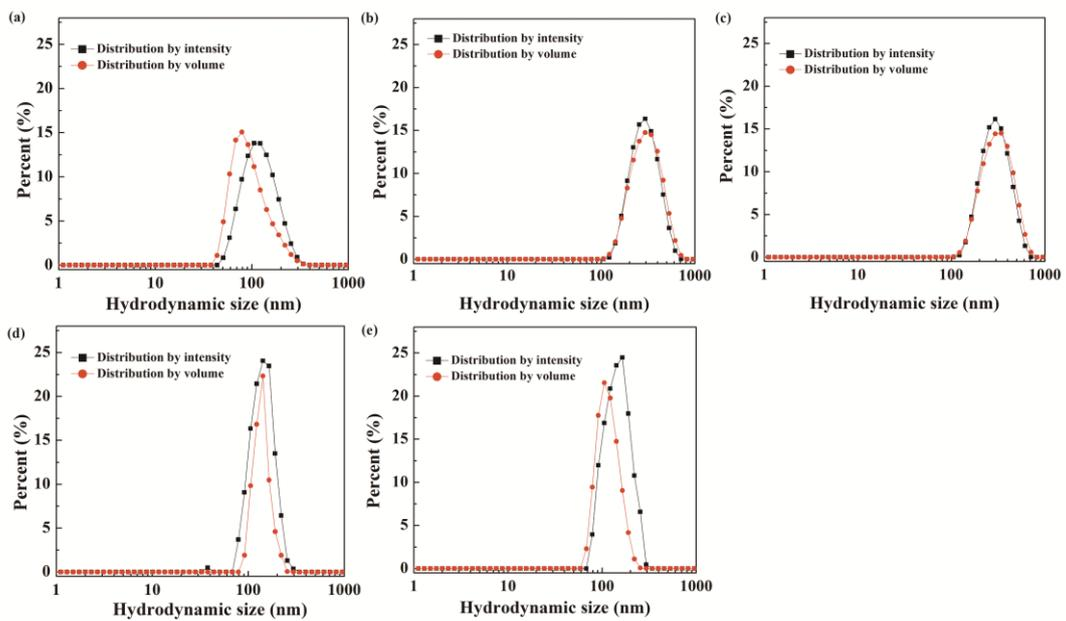
Fig.S6 Hydrodynamic size distributions of the (a) Fe<sub>3</sub>O<sub>4</sub> NPs, (b) LAP-Fe<sub>3</sub>O<sub>4</sub>, (c) LAP-Fe<sub>3</sub>O<sub>4</sub>@PDA, (d) LAP-Fe<sub>3</sub>O<sub>4</sub>@PDA-mPEG and (e) LAP-Fe<sub>3</sub>O<sub>4</sub>@PDA-PEG-PBA NPs measured by intensity and volume, respectively.
