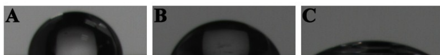
Fig. S5. Contact angle measurement of (A) bare Au, (B) Ab/Au, (C) Ab/MCH/PEG/Au surfaces.
