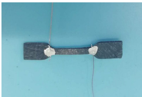
Fig. S9 Photo showing a strain sensor made of dumbbell specimen of G1.1 composite.
