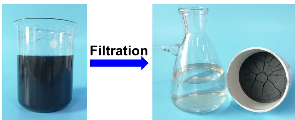
Fig. S1 Photo showing the unattached GNPs and ethanol could be easily separated from filtering fluid using filter paper.
