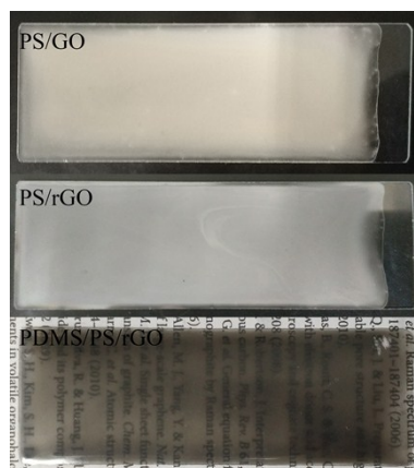
Figure S1. Optical images at different stages of the PDMS/PS/rGO sensor preparation process.
