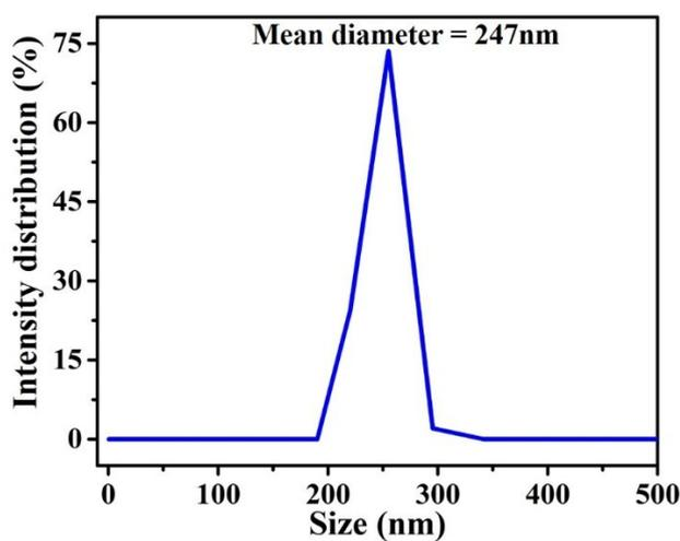
Fig. S4 The size distribution of BNNS measured by dynamic light scattering.
