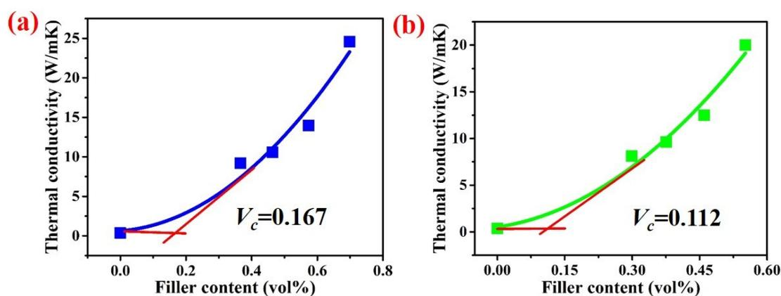
**Fig. S9** The tangent process of experimental data for (a) BNNS@PDA/PVA and (b) BNNS/PVA films to obtain  $V_c$ .
