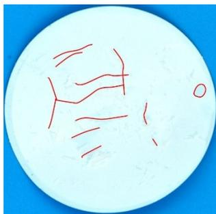
**Fig. S1** Digital photograph of BNNS/PVA film with the 75 wt% BNNS after slight bending. The red lines represent the cracks on the surface.
