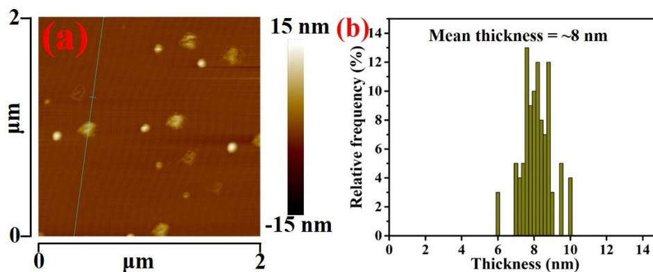
**Fig. S3** (a) More AFM images of BNNSs and (b) the distribution of thickness of BNNSs obtained by the statistical calculation.
