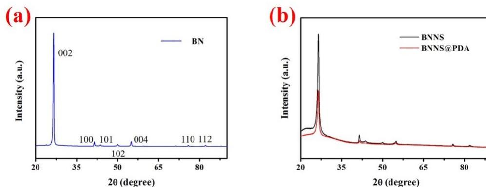
**Fig. S6** XRD patterns of (a) BN, BNNS and (b) BNNS@PDA.
