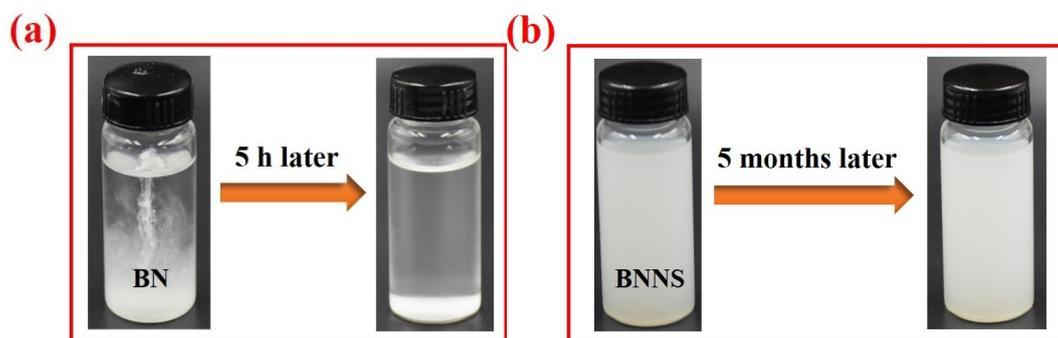
**Fig. S8** Optical images of (a) BN and (b) BNNS aqueous dispersion.
