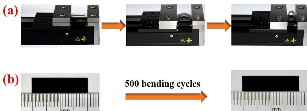
**Fig. S12** Optical images of (a) a whole bending process and (b) the 70 wt% BNNS@PDA/PVA film before and after 500 bending cycles.
