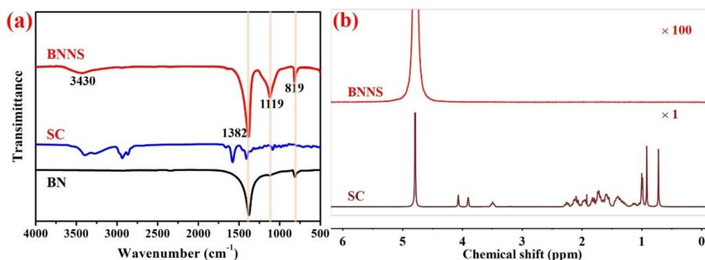
**Fig. S7** (a) FTIR spectra of BNNSs, SC and BN platelets; (b)  $^1\text{H}$ -NMR spectra of SC and BNNSs.
