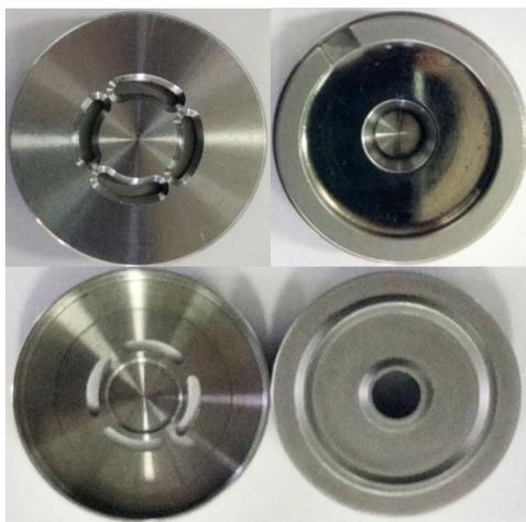
**Fig. S2** The special accessory used to measure the in-plane diffusivity.
