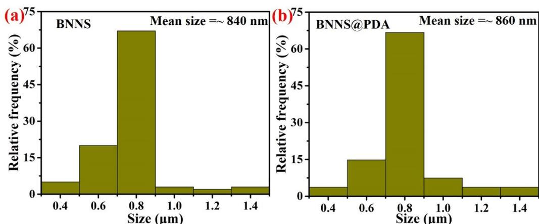
**Fig. S11** The distribution of size of BNNSs and BNNS@PDA obtained by the statistical calculation.
