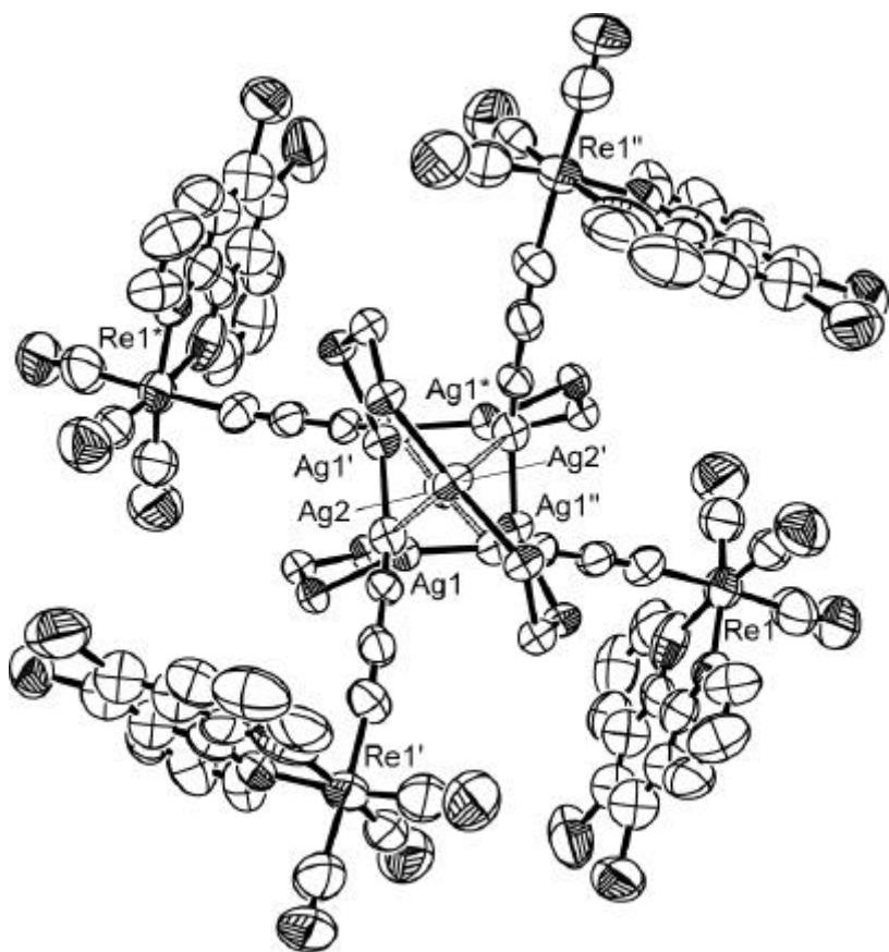
Perspective drawing of the complex cation of **4** with atomic numbering scheme. Hydrogen atoms and phenyl rings have been omitted for clarity. Thermal ellipsoids are shown at the 30% probability level.
