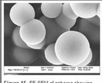
Figure 4S. FE-SEM of spheres showing fused spherical particles. Scale bar 200 nm.
