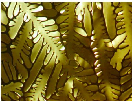
**Figure S1b.** Polarized optical micrograph of compound **6b** (200x) at 210° C.
