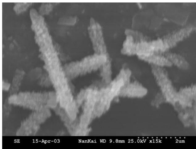
Fig.S3 SEM image of the rod-like ZnO mixed with \text{Zn}(\text{OH})_4^{2-} solution before the hydrothermal reaction, indicating the fast nucleation on the rod-like ZnO occurs prior to the hydrothermal reaction.
