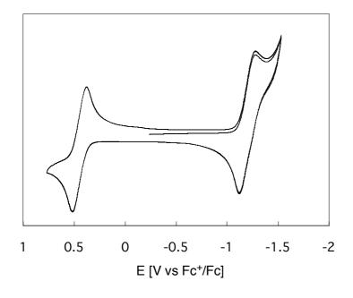
Cyclic voltammogram of **4** (multiple scan between -1.53 V and +0.77 V): 0.1 M Bu<sub>4</sub>NPF<sub>6</sub> in CH<sub>2</sub>Cl<sub>2</sub> at 24 °C with a Pt working electrode. Scan rate = 300 mV/s.
