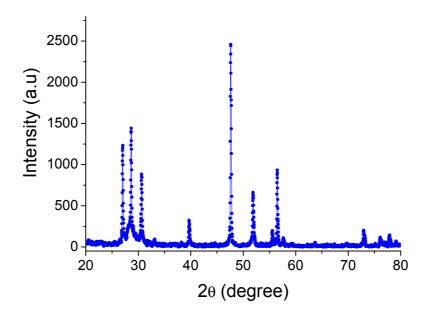
XRD of the ZnS nanobelt. It can be indexed to the wurtzite ZnS (JPCDS card 79-2204)
