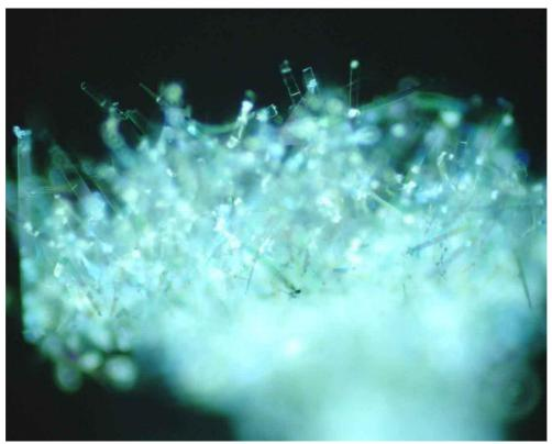
Photoluminescence microscopic image of the ZnS nanobelts under the excitation of 380 nm ultraviolet light.
