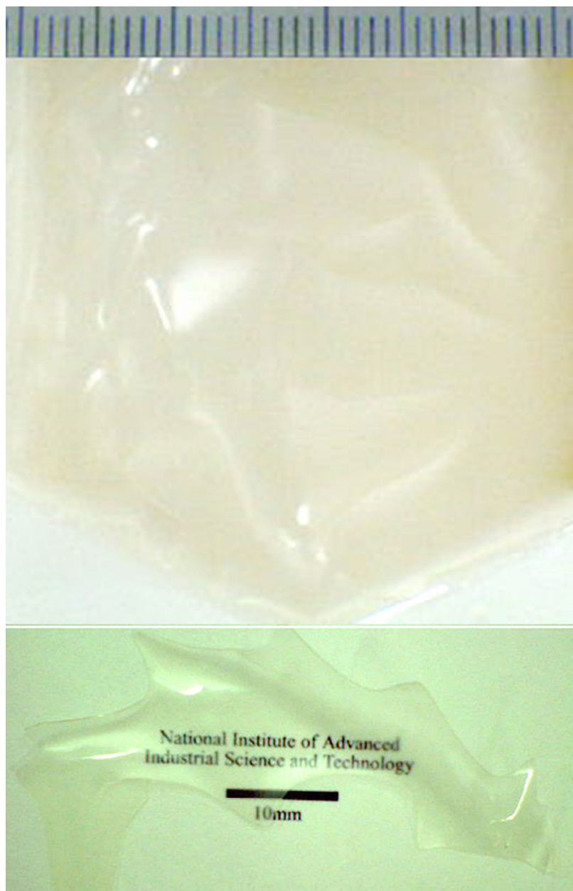
Fig. S3. Optical images of a self-standing 85- \mu\text{m} -thick film of mesostructured \text{TiO}_2\text{-P}_2\text{O}_5 after drying at 70^\circ\text{C} in air for 20 h (EISA was performed at 15^\circ\text{C}/80\%RH in air for 48 h).
