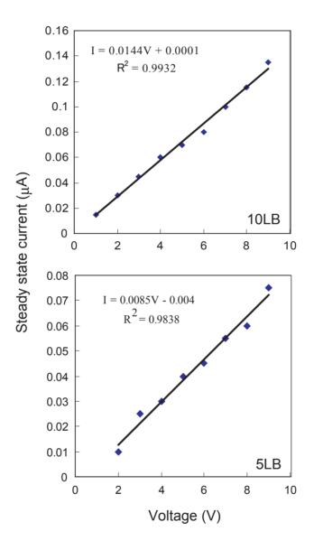
Results of DC measurements of 10- and 5-layered LB films after the photo-modification where the AC plots stayed constant. The Ohmic current was obtained in the 0-10 voltage region. The registivity of 69 M $_{\Omega}$  (10-layered LB film) and 125 M $_{\Omega}$  (5-layered LB films) conincided well with the R components in the AC measurements.
