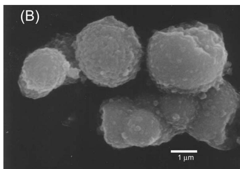
Supporting Information 1. TEM (A) and SEM (B) photographs of Cu/Mo-CTAB-3.1. In the TEM image a and b are basal and side views for stacked MoO<sub>2</sub>, respectively.
