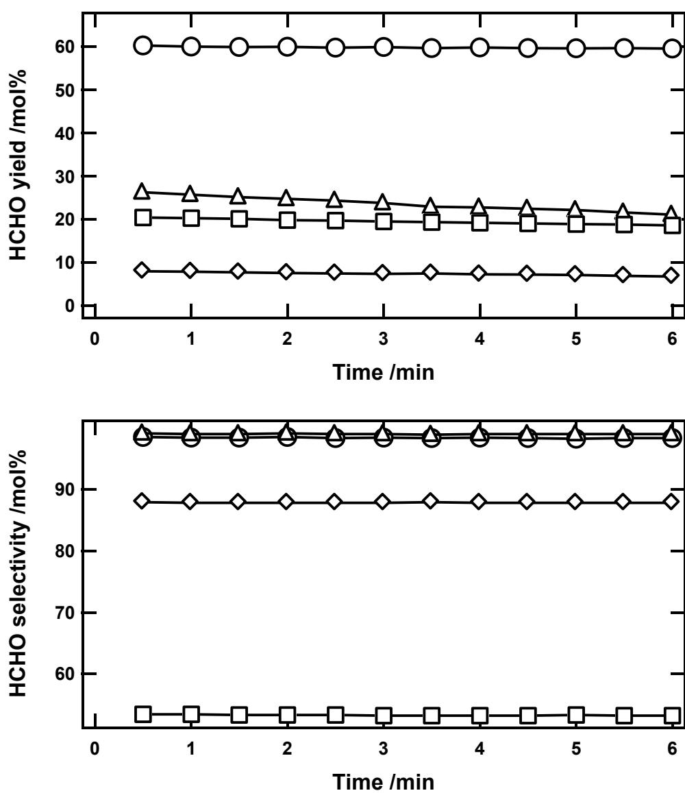
Supporting Information 2. HCHO yields and selectivities for the Cu nanoclusters supported on metal oxides. ○: Cu/Mo-CTAB-3.1, △: Cu/Zn-CTAB-3.7, ◇: Cu/Si-CTAB-4.3, and □: Cu/Al-CTAB-5.3.
