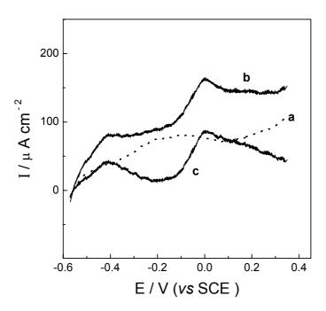
The current-potential curves obtained on a graphite-PTFE composite film electrode supported on glass carbon during the positive-going linear potential scan in (a) blank medium and (b) the culture of the electrochemical *E. coli* of generation II. The experiment was carried out at  $33^{\circ}$ C with potential scan rates of 10mV s<sup>-1</sup>. The curve (c) is obtained by subtracting of curve (b) with curve (a).
